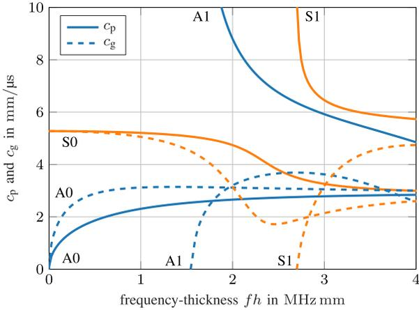
**Fig. 2.** Symmetric (S) and anti-symmetric (A) Lamb waves in an isotropic steel plate: the phase velocities  $c_p$  and group velocities  $c_g$  depend on the frequency-thickness product  $fh$ . Density:  $\rho = 7900 \text{ kg/m}^3$ , and Lamé parameters:  $\lambda = 115 \text{ GPa}$  and  $\mu = 76.9 \text{ GPa}$ .
