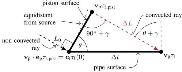
Fig. 5. Comparison of geometry of the two flow meters and the ray paths therein. The shown quantities are dependent on the mean flow velocity  $\bar{v}_0$ .
