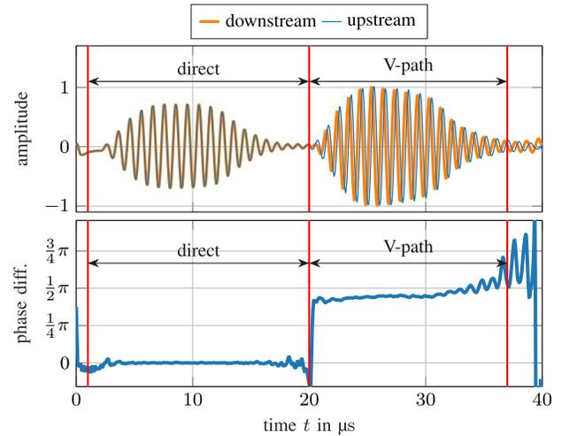
**Fig. 12.** Example of recorded ultrasonic upstream and a downstream signals at 6021 L/h and 19.9 °C.
