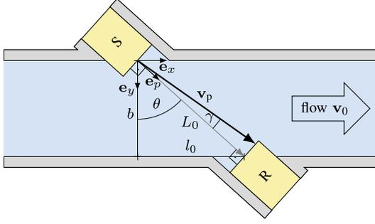
Fig. 4. Cross-sectional geometry of the wetted piston transducer-based flow meter. S: sender, R: receiver,  $\theta$ : radiation angle,  $\mathbf{e}_i$ : directional vectors,  $\mathbf{v}_0$ : flow velocity,  $\mathbf{v}_p$ : convected ray velocity,  $\gamma$ : convection angle, and  $l_0$ ,  $L_0$ , and  $b$ : geometric dimensions as indicated.
