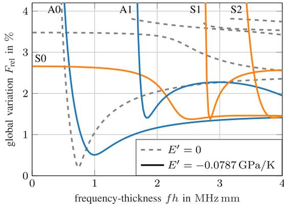
**Fig. 10.** Global root-mean-square relative variation  $F_{\text{rel}}$  of the meter's convection coefficient  $C$  due to temperature as defined in (16). A steel pipe with temperature-dependent Young's modulus (solid lines) is compared to the case where constant phase velocities are assumed (dashed lines). For piston transducer meters, the corresponding temperature variation is  $F_{\text{rel}} = 7.8\%$ .
