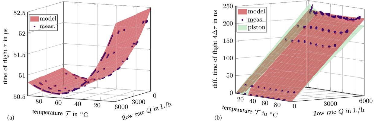
Fig. 13. Measurement compared to the model: the acquired (a) absolute and (b) differential time of flights match well with the temperature and flow rate-dependent model developed for Lamb wave-based flow meters. The corresponding behavior of piston transducer setups is also shown in (b) and expects a considerably larger variation with temperature.
