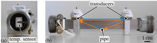
**Fig. 11.** Prototype in (a) front view and (b) lateral view. The transducers send alternately upstream (blue) and downstream (orange). The temperature sensor serves as reference only.
