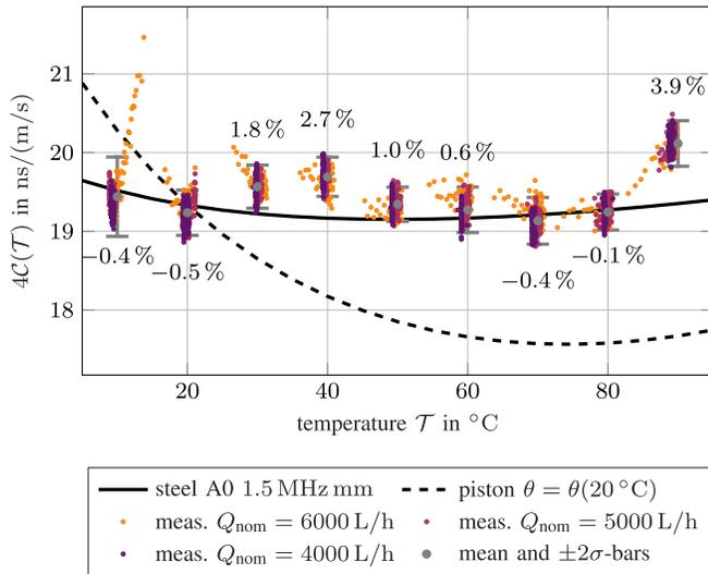
Fig. 14. Measured flow meter's convection coefficients  $C(T)$  in the turbulent regime compared to the model. The relative deviation to the model is indicated. The Lamb wave-based meter model is compared to the behavior expected for a conventional piston transducer device.
