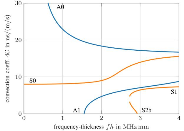
**Fig. 3.** Lamb wave-based UFM with a steel pipe: convection coefficients for water metering. Speed of sound:  $c_f = 1480 \text{ m/s}$  and  $b = 1.5 \text{ cm}$ .
