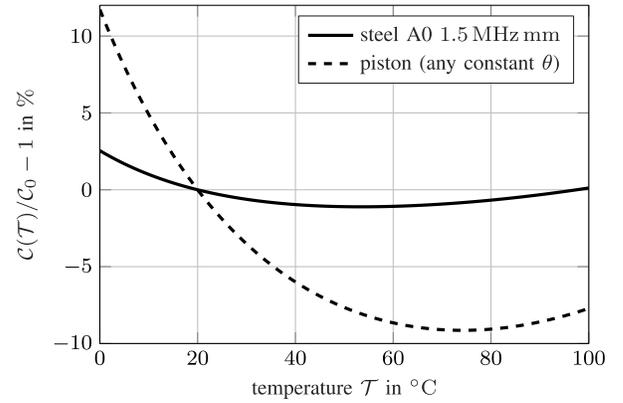
Fig. 9. Relative change with temperature of the convection coefficients  $\mathcal{C}$  of a Lamb wave-based flow meter compared to a conventional piston transducer device. The different behavior is due to the temperature-dependent radiation angle  $\theta$  of Lamb wave-based meters.
