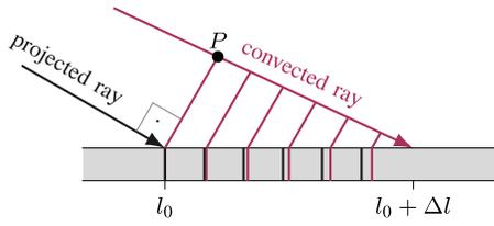
Fig. 6. Projected versus convected ray: the latter arrives earlier at  $l_0 + \Delta l$  as it is convected longer.
