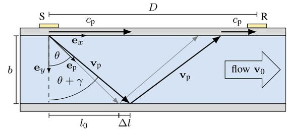
Fig. 1. Cross-sectional geometry of the Lamb wave-based flow meter. S: sender, R: receiver,  $c_p$ : phase velocity,  $\theta$ : radiation angle,  $e_r$ : directional vectors,  $v_0$ : flow velocity,  $v_p$ : convected ray velocity,  $\gamma$ : convection angle,  $\Delta l$ : convection distance, and  $l_0$ ,  $b$ , and  $D$ : geometric dimensions as indicated.
