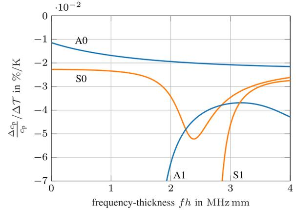
Fig. 8. Lamb waves in steel: relative change in phase velocity per unit change in temperature with respect to 20 °C.
